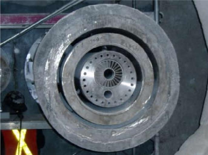
Developed using CFD modelling, the DFN (direct-fired nozzle) burner has been proven across many projects to provide outstanding improvements in areas such as production, fuel consumption, NOx emissions, and ash ring formation.
